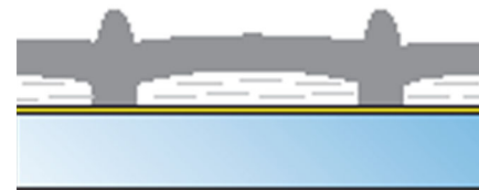
This cross-section diagram shows how Philips’ prototype liquid crystal display was made. When researchers exposed a mix of liquid crystals and plastic to ultraviolet light, the plastic hardened into pixel-size cells that contained the liquid crystals.
