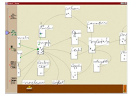
The Denim tool allows Web designers to build working Web sites by roughly drawing pages and the links among them.
