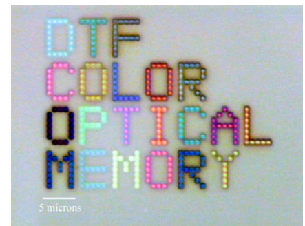
These colored letters are formed by holes in the thin film storage media. The colored pixels can also be used to store 4-bit digital data.
