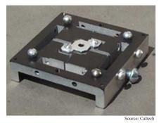
The springs are not visible in this photograph of a vision sensor, which measures slightly more than one inch square. The lense is under the light-colored piece of metal in the center of the device.
