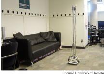
This museum guide robot navigates by pinpointing the sound of its own voice using a series of microphones placed around the room.
