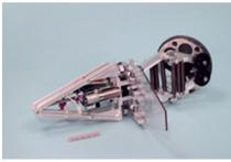
Source: JPL/Caltech The frogbot's spring-loaded leg allows it to hop relatively quickly across rough terrain. The latest version, not shown, includes wheels for rolling short distances.
