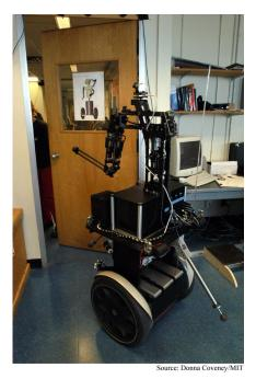
This robot, which combines a mechanical arm with a modified version of the Segway scooter, is capable of finding doors and pushing them open.
