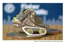
This microrobot is parked on a quarter. The robot's treads help it traverse rough terrain like carpet.
