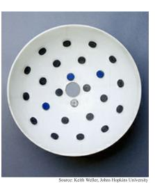
The ball is lined with a series of permanent magnets.
