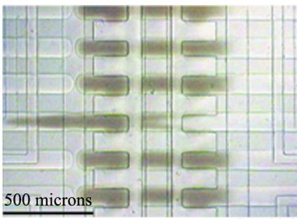
These close-ups of a second rubber chip show two fluids filling chambers in separate columns, the filled chambers, the fluids mixing, and the mix being purged from the chip.
