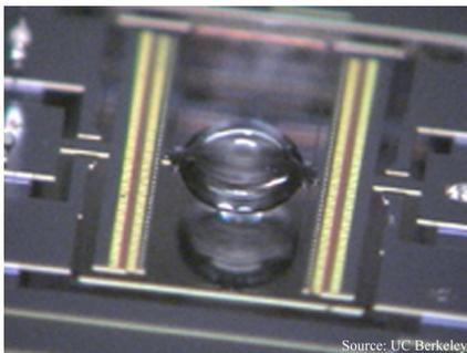
This stacked pair of lenses measures one-third of a millimeter across -- small enough to foster microscopes capable of imaging individual cells working inside the body. The metal strips bracketing the top lens are microactuators that focus the lenses.
