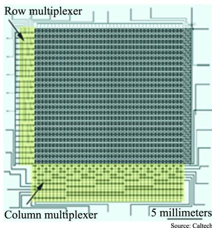
The grid in the center of this rubber chip contains 1,000 tiny chambers, which can each hold about one 80th of a drop of water. A pair of multiplexers control the flow of fluid through the chip, allowing each chamber to be accessed individually.
