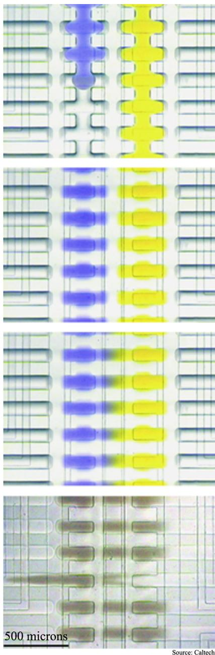
These close-ups of a second rubber chip show two fluids filling chambers in separate columns, the filled chambers, the fluids mixing, and the mix being purged from the chip.
