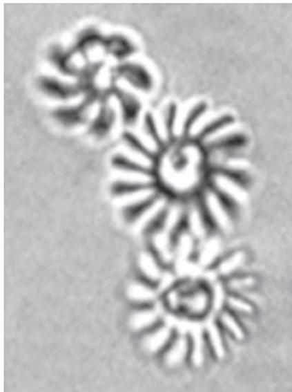
By moving the photosensitive resin around in the light the researchers were able to create three-dimensional objects. Once an object was finished, they used acetone to dissolve the remaining liquid resin.
