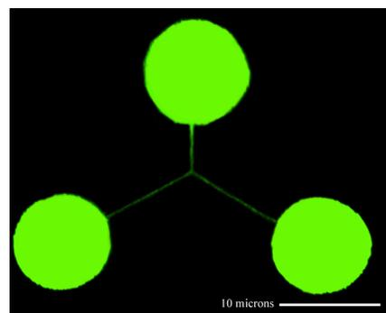
Three artificial cells, each twice the size of a red blood cell, are linked via nanotubes.
