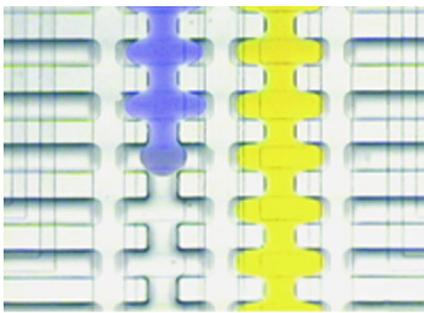
adding a fluid that becomes fluorescent in the presence of a particular enzyme. This allowed the researchers to determine which bacteria produced the enzyme.
