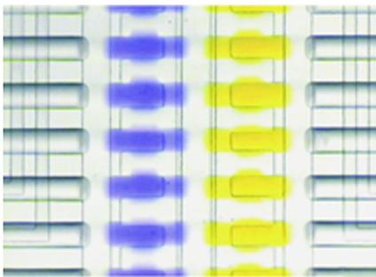
There are limitations to the rubber chips, according to Quake. Some liquids, like certain organic solvents, can break down the chip's rubber material, and there is a danger of contamination from molecules diffusing through the walls of the chambers and channels. There is also a possibility that some molecules will stick to the walls after the chip's contents have been emptied.
