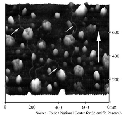
The smaller arrows point to string-like DNA molecules. The clumps are carbon fibers. When metal electrodes on both ends of the DNA strands are cooled to the point of superconductivity, the electrical resistance in the strands decreases dramatically.
