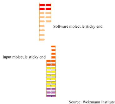
The short, artificially-constructed DNA molecules depicted here can carry out computational steps by matching and joining the exposed bases, or sticky ends.
