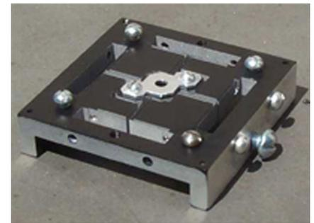
The springs are not visible in this photograph of a vision sensor, which measures slightly more than one inch square. The lens is under the light-colored piece of metal in the center of the device.
