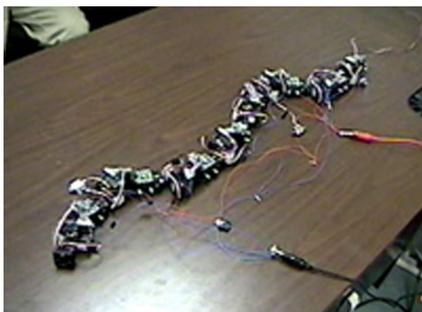
The first video shows an insect-like robot doing a push-up. The second video shows a robot moving like a snake. The interchangeable modules that make up these robots communicate via a hormone-like messaging system to coordinate their movements.
