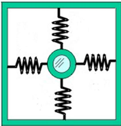
This diagram depicts a vision sensor for robots. The sensor uses springs to vibrate a lens in order to increase its resolution.
